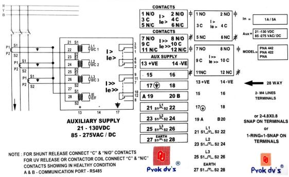
Note: Do Not Connect Terminals 19 & 20 (A& B Of Rs 485) For Hv Test RS 232 Port is provided on the front facia
